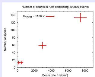
For a give gain the sparking probability is linear with the beam rate till  $8000 \text{ Hz}/\text{cm}^2$  (our measurable limit).
