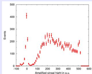
The distortion at the tail of the Landau distribution is made by the electronics which does not need high dynamic range at the final design.
