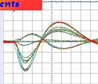
Dividing the correlated signal into categories: below or above threshold, these effect become measurable. Negative correlations shows the expected tendency, positive correlations have huge error-bars due to the big fluctuations in the tail of the Landau distribution, however slightly increase can be observed.
